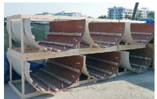
Galvashield DAS Jackets Prior to Installation
