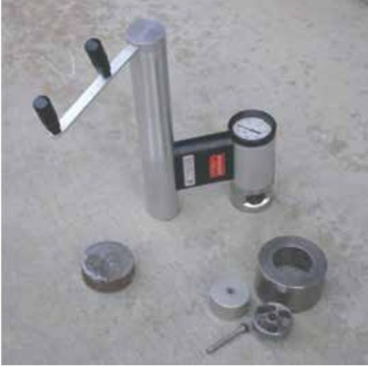
Fig. 2: Pull-off bond testing equipment
