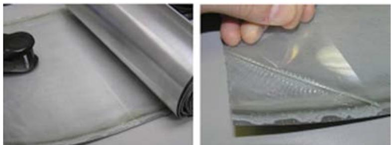
Fig. 10: Surface-applied galvanic metalizing system
