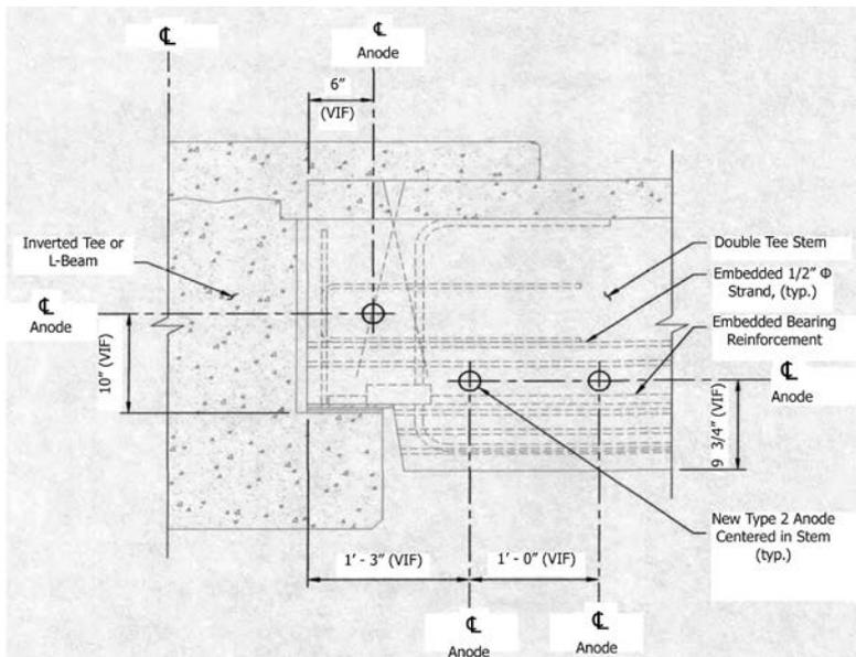
Fig. 13: Discrete galvanic Type 2 anodes protect T-stem end
