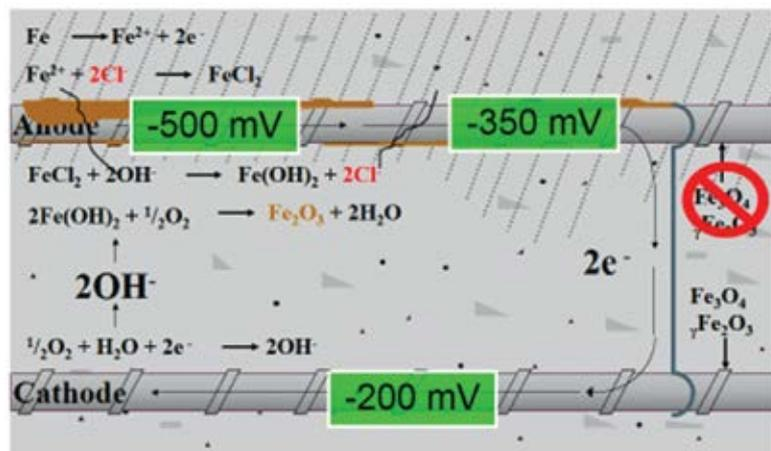
Fig. 2: Reinforcing steel corrosion cell in concrete
