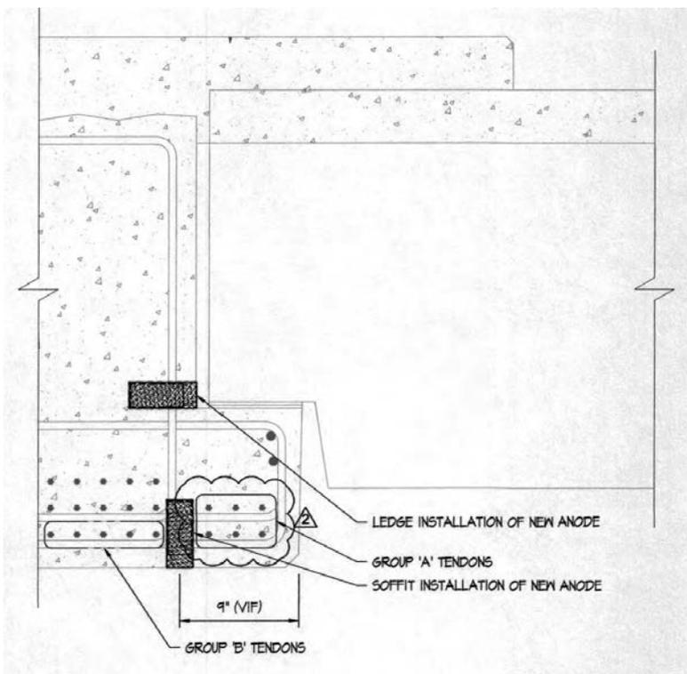
Fig. 14: Discrete galvanic Type 2 anodes provide corrosion protection at inverted T-beam haunch
