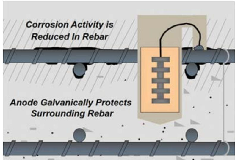
Fig. 9: Discrete galvanic Type 2 anode
