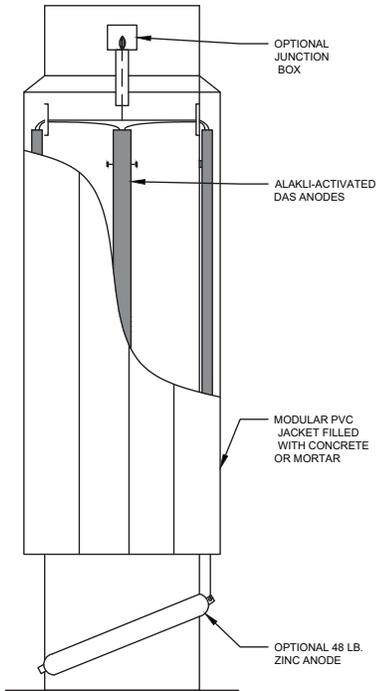
An electrical connection must be made to the reinforcing steel that is to be protected. Electrical connection can be made to exposed reinforcing steel. If no exposed steel is present, a concrete excavation will be required to make the reinforcing steel connection. In order for the system to work properly, the steel reinforcement must be electrically continuous. If not, electrical continuity must be established.
