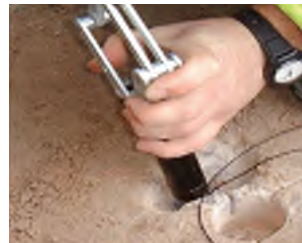
5 Pop rivet installation to steel
