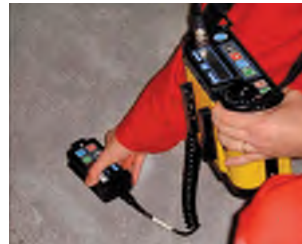
1 Locate steel and position anode
