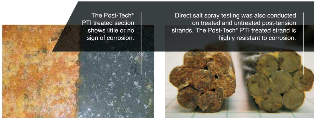
The Post-Tech® PTI treated section shows little or no sign of corrosion.
