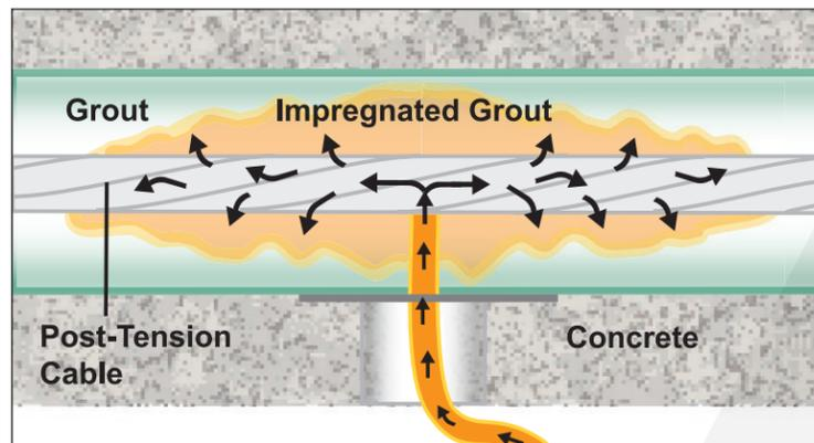
Illustrations of Post-Tech® PTI Impregnation System being completed from the end of the tendon and from an intermediate location.
