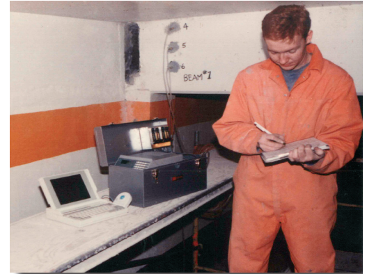
Post-Tech PT Corrosion Evaluation of Cables
