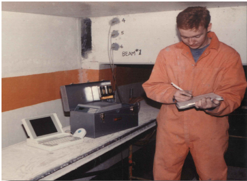
Post-Tech PT Corrosion Evaluation of Cables
