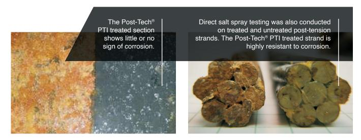
Salt spray testing on steel plate with untreated (left) and Post-Tech® PTI treated section (right).
