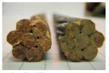
Post-Tech PTI impregnation material mitigates corrosion on post-tension strands (right)
