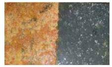
Salt spray testing on steel plate with Post-Tech PTI treated section (right)
